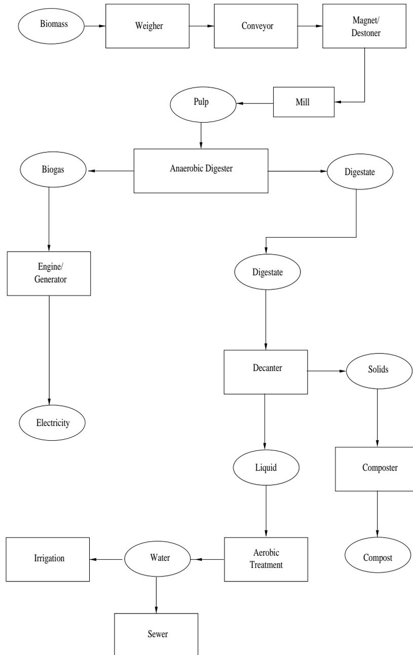
Fig. 6. Flow sheet for the AD of biomass.
