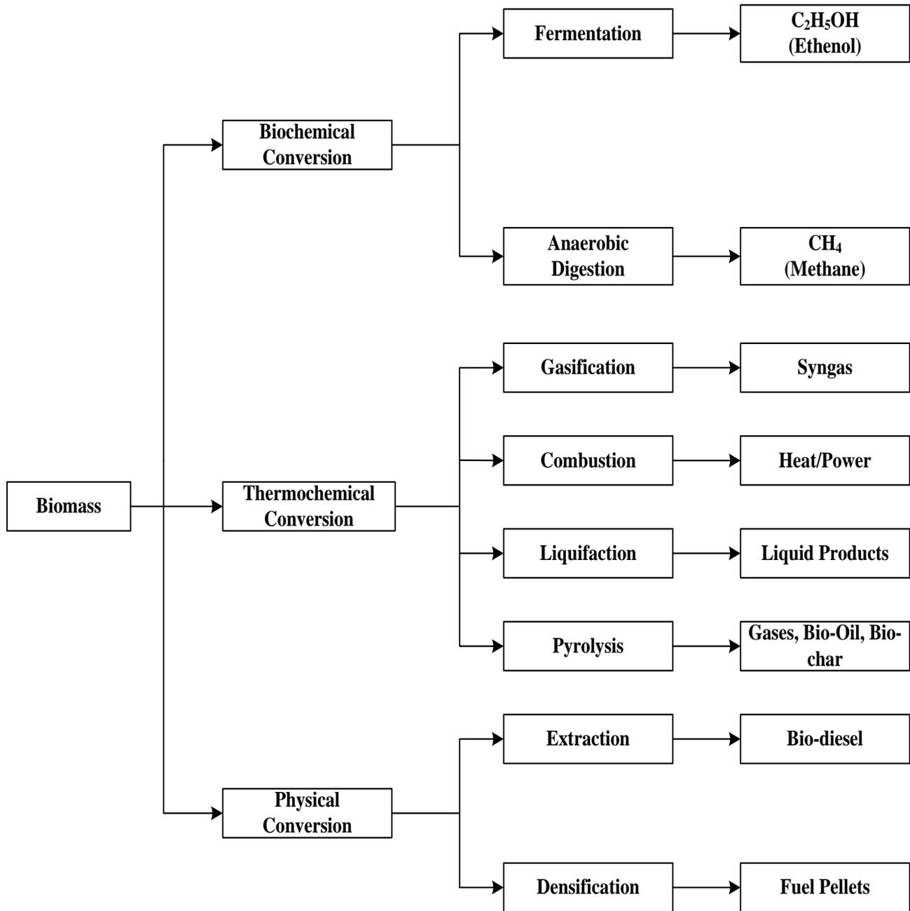
Figure-1: Conversion technologies for biomass into energy.
